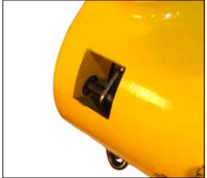
Figure 7-12. Removing Chain Guide Support Pins
