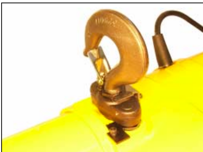
Figure 7-15. Removing Upper Hook and Hook Nut from Hoist Frame (1/4 through 1 Ton Models)
