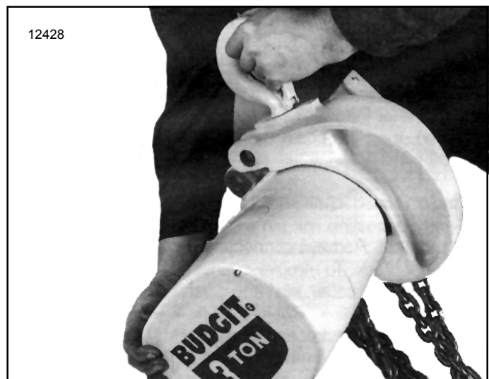
Figure 7-2. Removing 3 Ton Hanger Bracket from Hoist Frame
