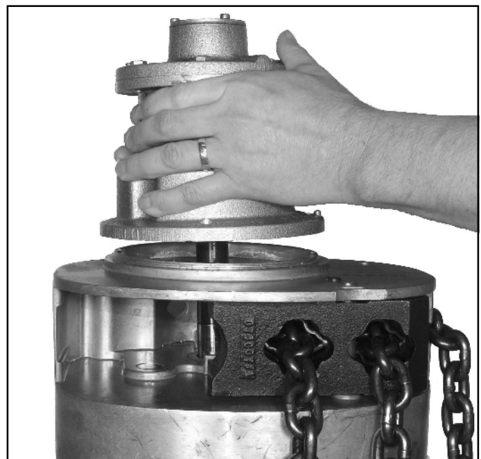
Figure 7-8. Removing Motor Assembly
